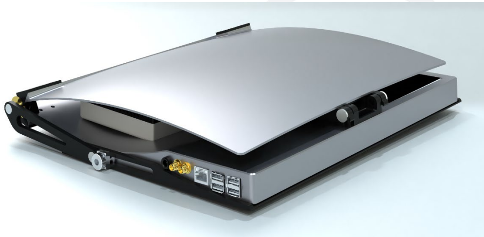
Figure 14: Folded reflector, the overall system package that is about 30x25x5 cm 3 .
