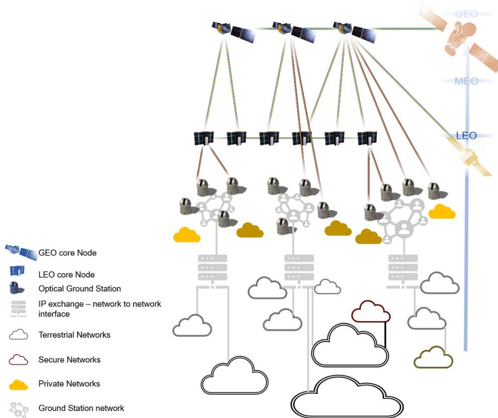
**Figure 1 Vision of a high throughput optical space network bringing high data rate terrestrial connectivity to multiple space users across different orbits (e.g., LEO, MEO, GEO) and to ground users located in remote areas with no available broadband access.**
