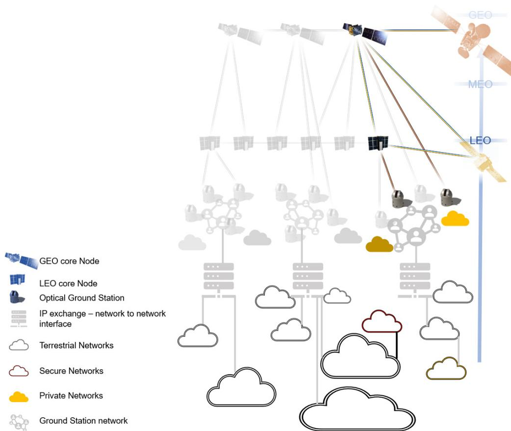
**Figure 2 Demo System mission of a downscaled high throughput optical space network (i.e., HydRON-DS), demonstrating key optical / digital technologies and validating operational concepts required for the HydRON vision.**
